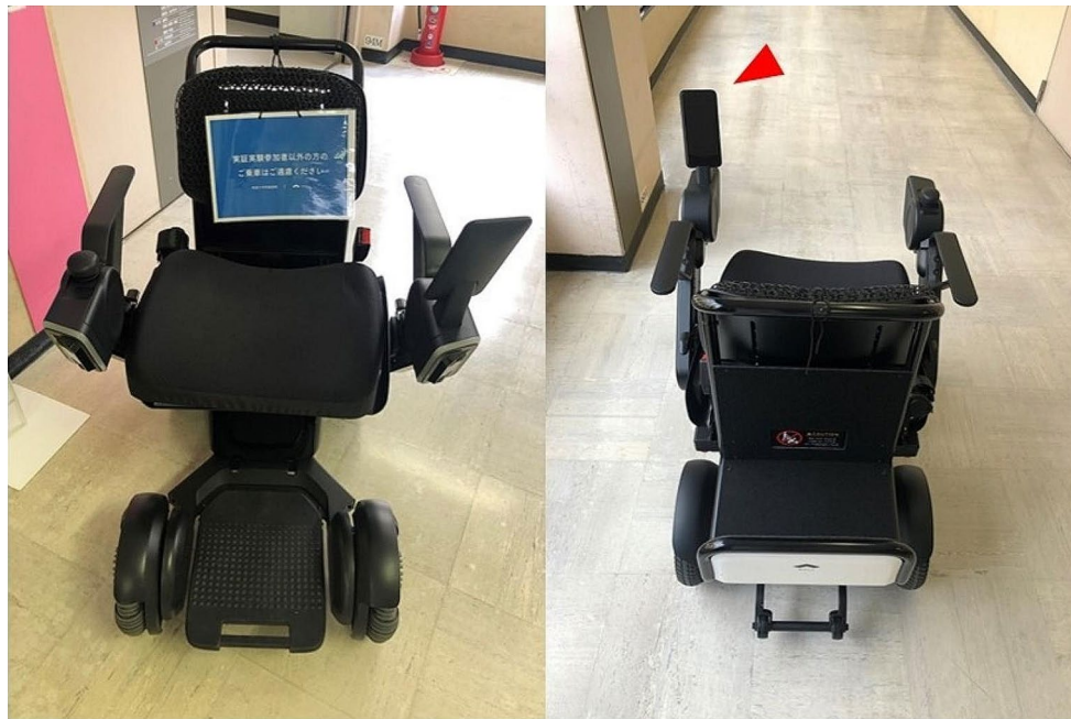
Fig. 1 The driverless mobility used in the present study is manufactured by WHILL Inc. The arrowhead indicates the tablet device for the user
